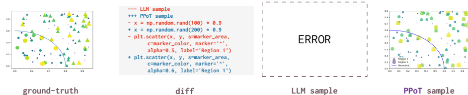
Figure 4: PPoT enables cheap samples that correct the LLM generated program. From left to right, we show the ground-truth plot, followed by a diff between the LLM and PPoT samples, the LLM sample rendering and then the resulting PPoT sample. The LLM generated code contains a runtime error and so produced no graph.
